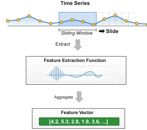
Fig. 2: Illustration of the sliding feature extraction process.
