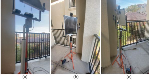
Fig. 4. Portable multi-axis solar tracking prototype for hardware validation. (a) Tracker raised by the linear actuator. (b) Actuation and mounting structure connecting the PV panel to the tripod (DC motor on the arm and stepper motor at the base). (c) Prototype oriented toward incident sunlight from a different viewing angle, illustrating multi-axis alignment capability.
