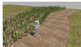
Fig. 1: Hunter biped in a Gazebo-simulated agricultural field with crop rows, exhibiting variable friction, wet or dry, and compliance typical of tilled soils.
