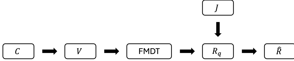
Fig. 1. From the circuit C , features V are extracted and evaluated via FMDT to obtain an intermediate ranking R_q , which is refined by considering J and using TOPSIS to produce the final ranking \hat{R} .
