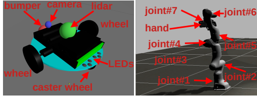
Fig. 1. Simulated robots. Left: two-wheeled 3\pi robot. Lidar sensors and camera objects are just visual placeholders to indicate their positions. Right: 7-d.o.f. Franka Emika Panda arm.
