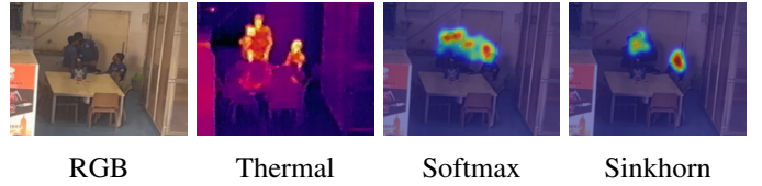
Fig. 6: Comparison of attention maps obtained using Softmax and Sinkhorn normalization.
