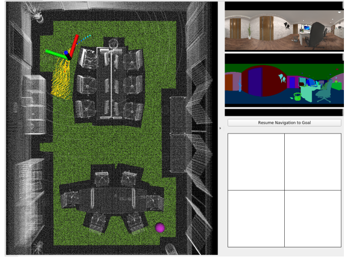
Fig. 6. Real-time visualization of the exploration process. The system builds a 2D grid map while simultaneously populating a 3D semantic voxel map for object grounding.
