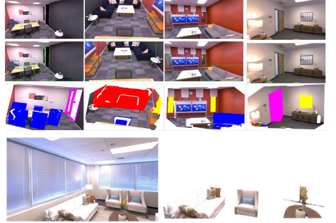
Fig. 3. Semantic object detection in reconstructed scenes. Top: Original RGB; middle: Detected objects (YOLO/VLM) with bounding boxes in 3D; bottom: Highlighted semantic objects.
