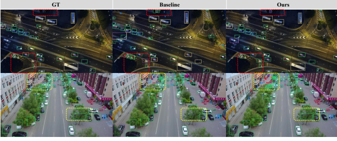
Fig. 3. Qualitative comparison of detection results on the VisDrone dataset. The first column shows the annotated images (ground truth), the second column presents the predictions of the baseline model D-FINE-N, and the third column shows the results of the proposed FA-DETR.
