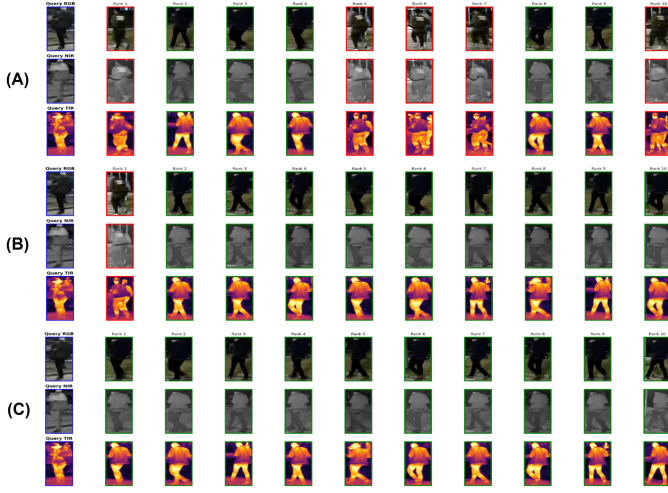
Fig. 8. Ranking list on person ReID. (A) Baseline. (B) Baseline + SIPC. (C) Full model. Green/red boxes indicate correct/incorrect matches.
