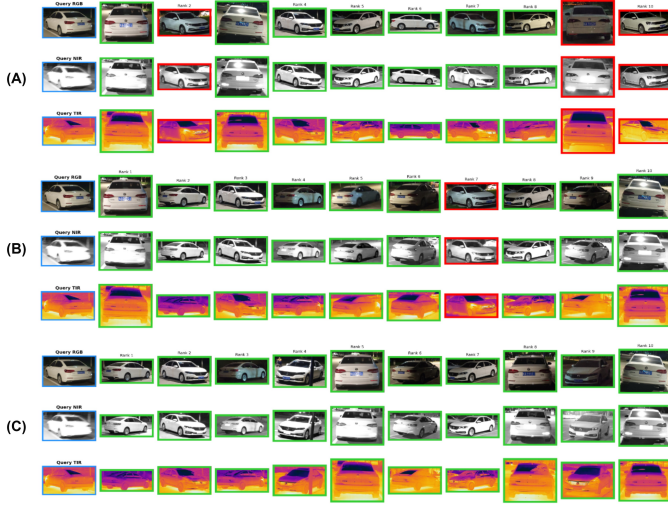
Fig. 9. Ranking list on vehicle ReID. (A) Baseline. (B) Baseline + SIPC. (C) Full model. Green/red boxes indicate correct/incorrect matches.
