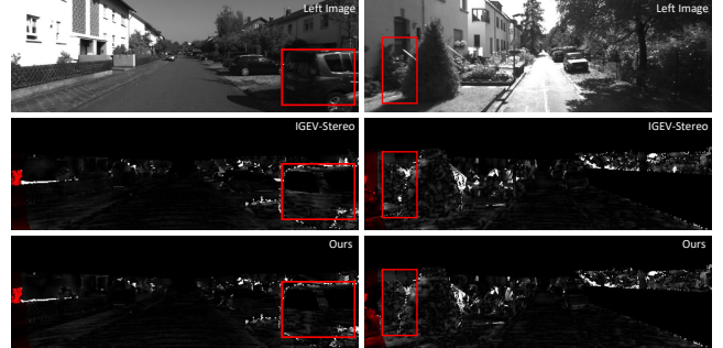
Fig. 6. Error-map comparisons on the KITTI 2012 test set. Black indicates accurate regions and white denotes large disparity errors. Red boxes highlight challenging areas such as object boundaries and weak-texture regions.
