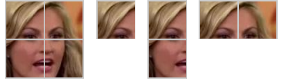
Fig. 2. When K = 2 , the pattern set contains 10 classes: four 1 \times 1 blocks, two 1 \times 2 rectangles, two 2 \times 1 rectangles, one 2 \times 2 full-coverage pattern, and one non-occluded pattern.
