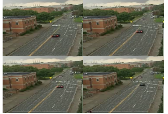
Fig. 4. Final flood simulation. The simulation generates physically consistent results, displaying wake formation behind vehicles and realistic, depth-dependent water opacity.
