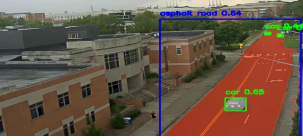
Fig. 3. Visualization of the Scene Decomposition module. Detected bounding boxes identify vehicles and guide the generation of precise segmentation masks, defining rigid obstacles used in our physics-based simulation.
