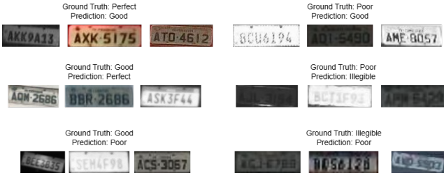
Fig. 5. Examples of misclassified LPs illustrating borderline legibility cases.
