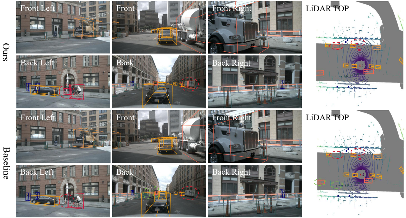
Fig. 4. Qualitative comparison of 3D detection results between FocusBEV (top) and the Baseline (bottom). Red dashed circles highlight targets missed by the baseline but successfully detected by FocusBEV. Green dashed circles indicate false positive predictions or orientation errors generated by the baseline in sparse areas.
