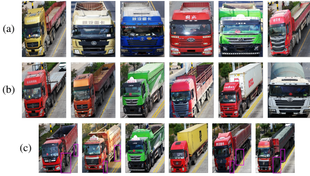
Fig. 1: Diversity in Truck Characteristics. (a) Diversity of fronts: different colors, models and manufacturers. (b) Diversity of carriages: flatbed, palletized, tipper, barn-rail, box, tank, respectively. (c) Diversity of axles: different axle numbers and axle configurations.
