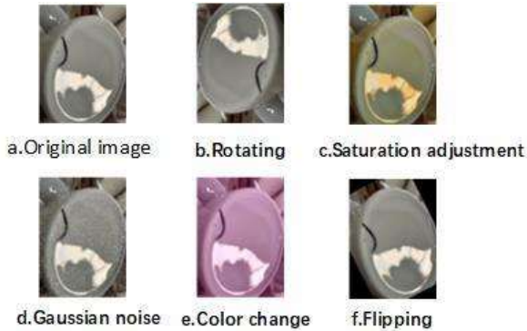
Fig. 7. Examples of data augmentation applied to the ceramic cup defect dataset
