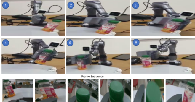
Fig. 11. Qualitative slanted-object grasps with MVB-Grasp in the real world.
