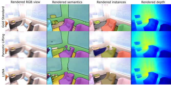
Fig. 5. Qualitative comparison of panoptic segmentation under strong motion blur. Top to bottom: ground truth, panoptic lifting, and our method LUNA. Panoptic lifting exhibits incomplete segmentation and semantic drift, with only partial detection of key objects (e.g., the chair). LUNA reconstructs complete object boundaries and sharper depth edges, demonstrating robustness from geometry-aware depth supervision and adaptive multitask optimization.
